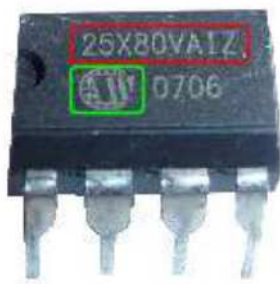
Manufacturer WINBOND (stylized "W") Type 25X80VAIZ Package design DIP-8 (2x4 Pins = 8 Pins)
