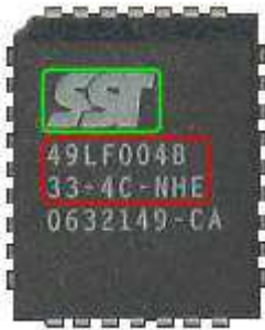
Manufacturer SST Type 49LF004B 33-4C-NHE Package design PLCC-32 (2x7 and 2x9 Pins = 32 Pins)
